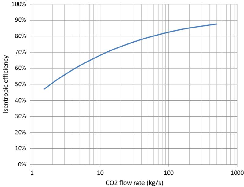
**Figure 6: Pump efficiency as a function of capacity, assuming high specific speed.**
