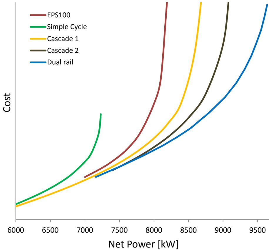
Figure 3: System cost versus power output, several candidate sCO<sub>2</sub> power cycle architectures
