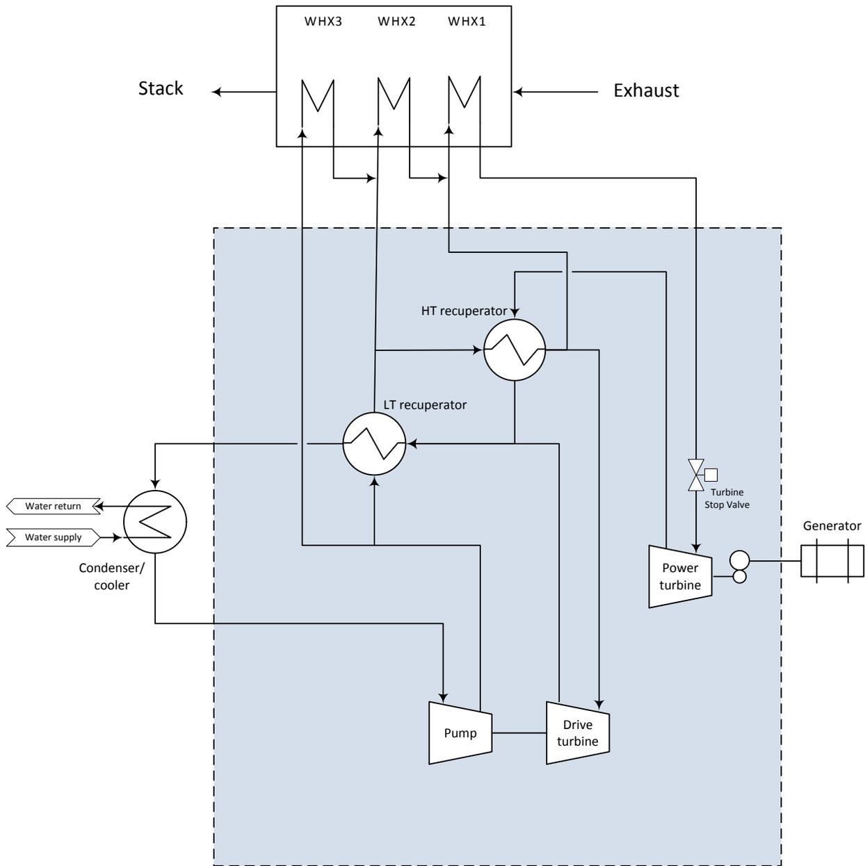
Figure 4: Dual rail cycle sCO<sub>2</sub> cycle.
