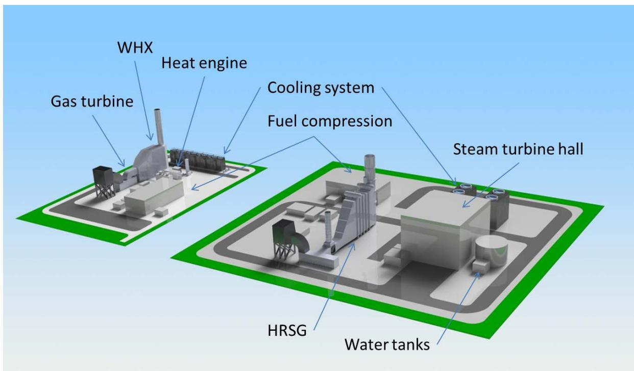
Figure 8: Comparison of LM2500/sCO<sub>2</sub> combined cycle installation with LM2500/HRSG
