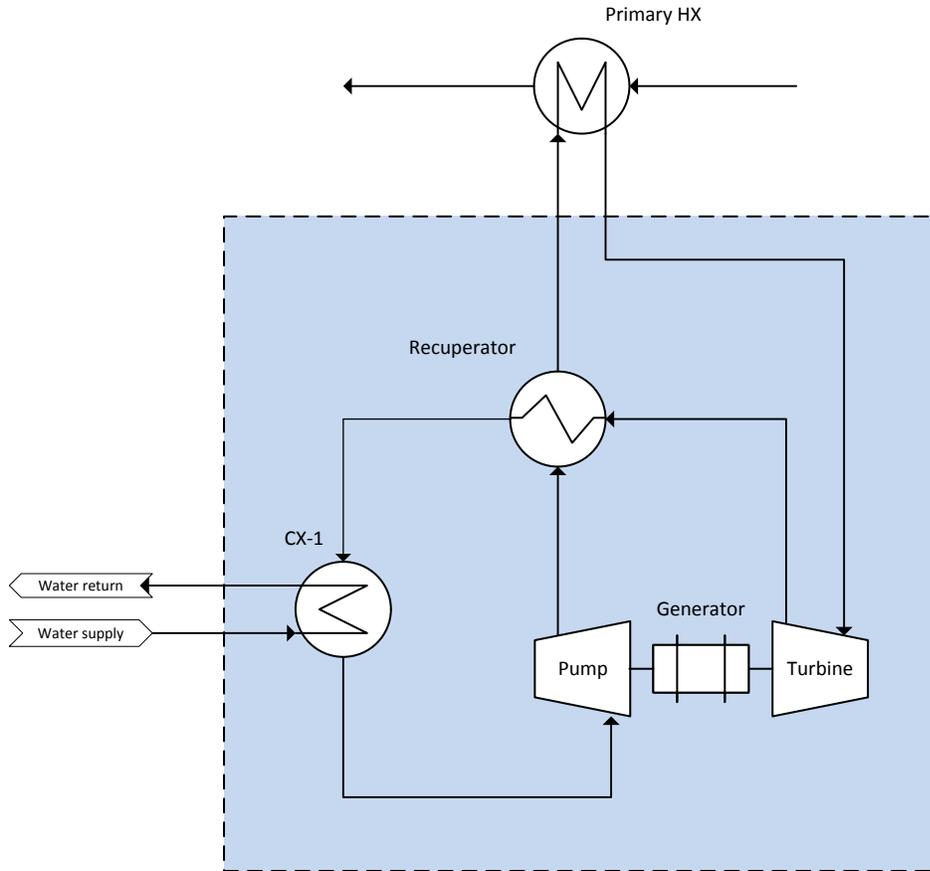
Figure 1: Simple recuperated sCO<sub>2</sub> cycle
