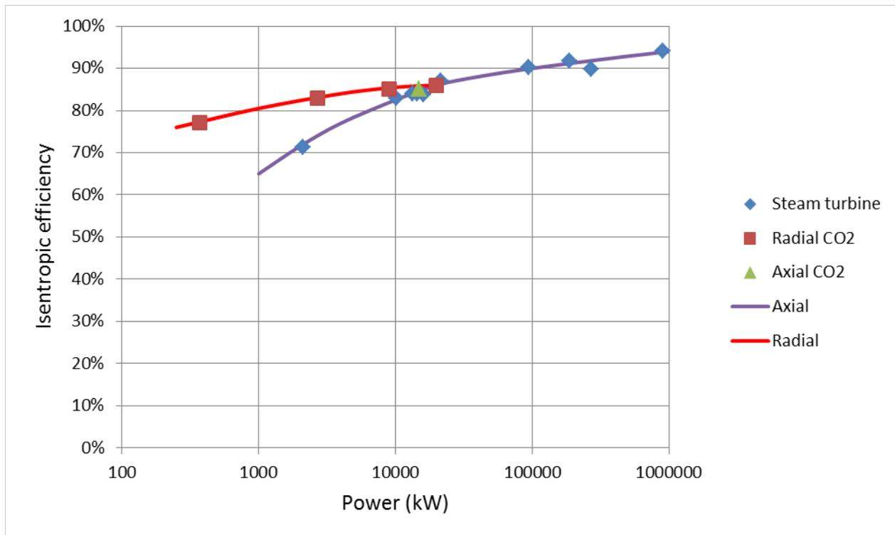
Figure 5: Turbine efficiency vs shaft power
