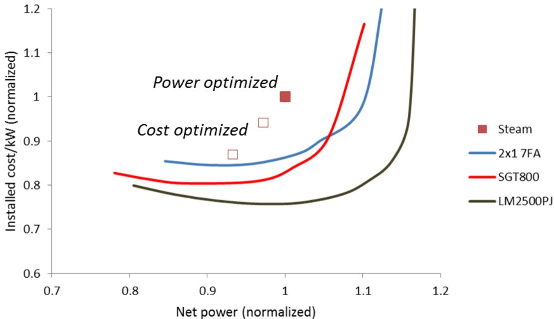
Figure 7: Cost/kW vs net power for three sizes of combined cycle plants, normalized to GT-Pro “power-optimized” cases. The open symbols are two example GT-Pro cases using the “cost-optimized” option.
