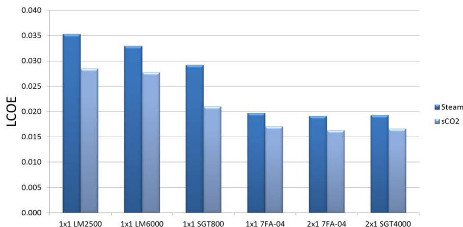
**Figure 10: Projected LCOE for bottoming cycle power generation, assuming 5% discount rate, 30 year plant life and 85% utilization factor for several sample applications.**
