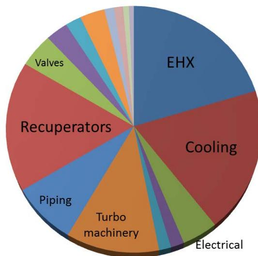
Figure 9: Selected approximate equipment cost breakdown for sCO<sub>2</sub> system
